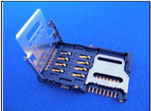
Step 6:Unlock MicroSD Metal-Cover
