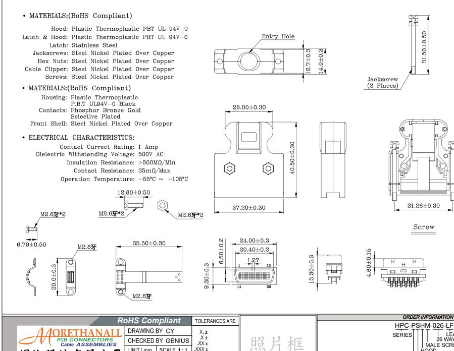
LEADFREE **26 WAY** MALE SCREW HOOD SOLDER 1.27mm(.050") Ribbon 26Pos DESCRIPTION: Cable Plug Connector Solder Assembly Type
