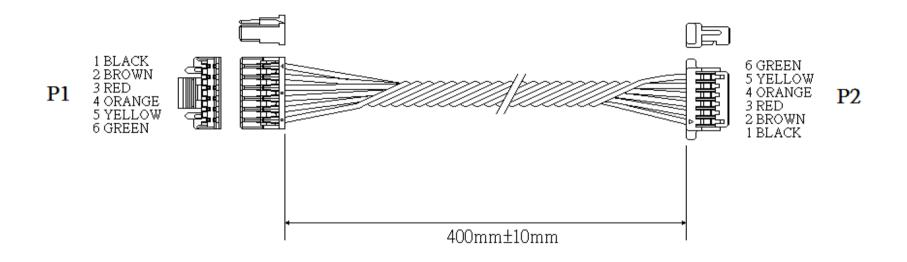
1. P1: 1.25mm PITCH CRIMP TERMINAL AND HOUSING GH-H-06 COLOR-WHITE
