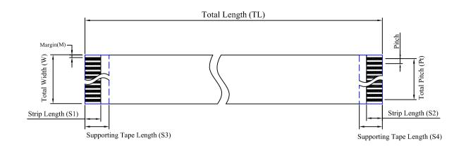
UL Style No : UL2896 /  $80^{\circ}$  C , 30V UL Marking on one side
