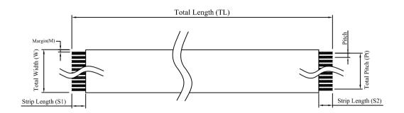
UL Style No: UL2643 / 105° C, 300V UL Marking on one side
