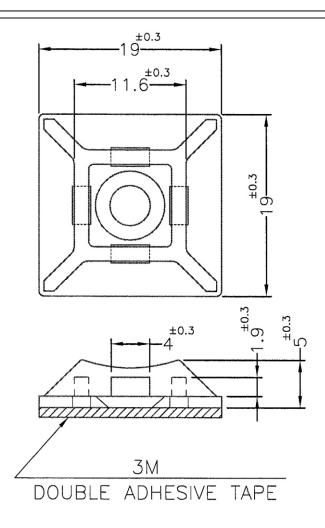
NOTE: 1. THE PRODUCT SIZE IS NOT INCLUDED THE SIZES OF ADHESIVE TAPE AND ITS LINER. 產品尺寸皆不含背膠及離型紙.
