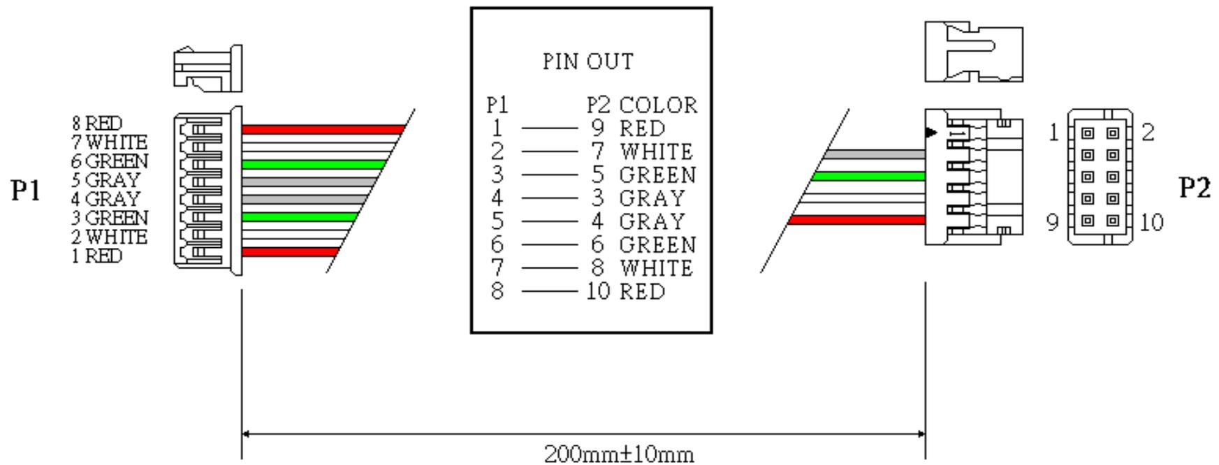
1. P1 : 1.25mm PITCH CRIMP TERMINAL AND HOUSING FH-H-08 COLOR=WHITE
